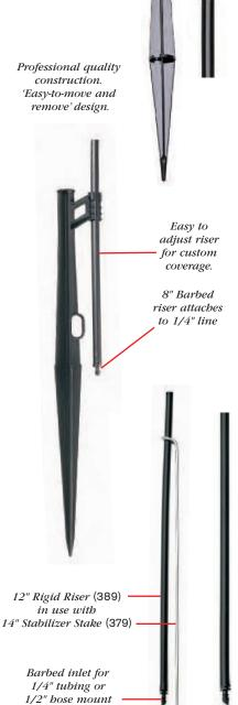
**8" Stakes for Low-Flow Sprinklers** Heavy duty 8" stakes with 4" risers for use with low-flow sprinklers, sprayers and jets. 1/4" double-barbed inlet secures connection of 1/4" tubing and directs it downward below soil surface for connection to 1/2" supply line. Constructed of high impact ABS and high density polyethylene.
