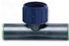
**3/4" Hose Thread Swivel x 1/2" Compression Tee** For use with 1/2" (.620"–.630" O.D.) hose only. Includes filter washer. *Color coded Green compression ring*
