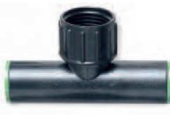
**3/4" Pipe Thread Swivel x 1/2" Compression Tee** For use with 1/2" (.620"–.630" O.D.) hose only. Washer included. *Color coded Green compression ring*
