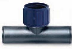
**3/4" Hose Thread Swivel x 5/8" Compression Tee** For use with 5/8" (.690"–.700" O.D.) hose only. Includes filter washer. *Color coded Black compression ring*
